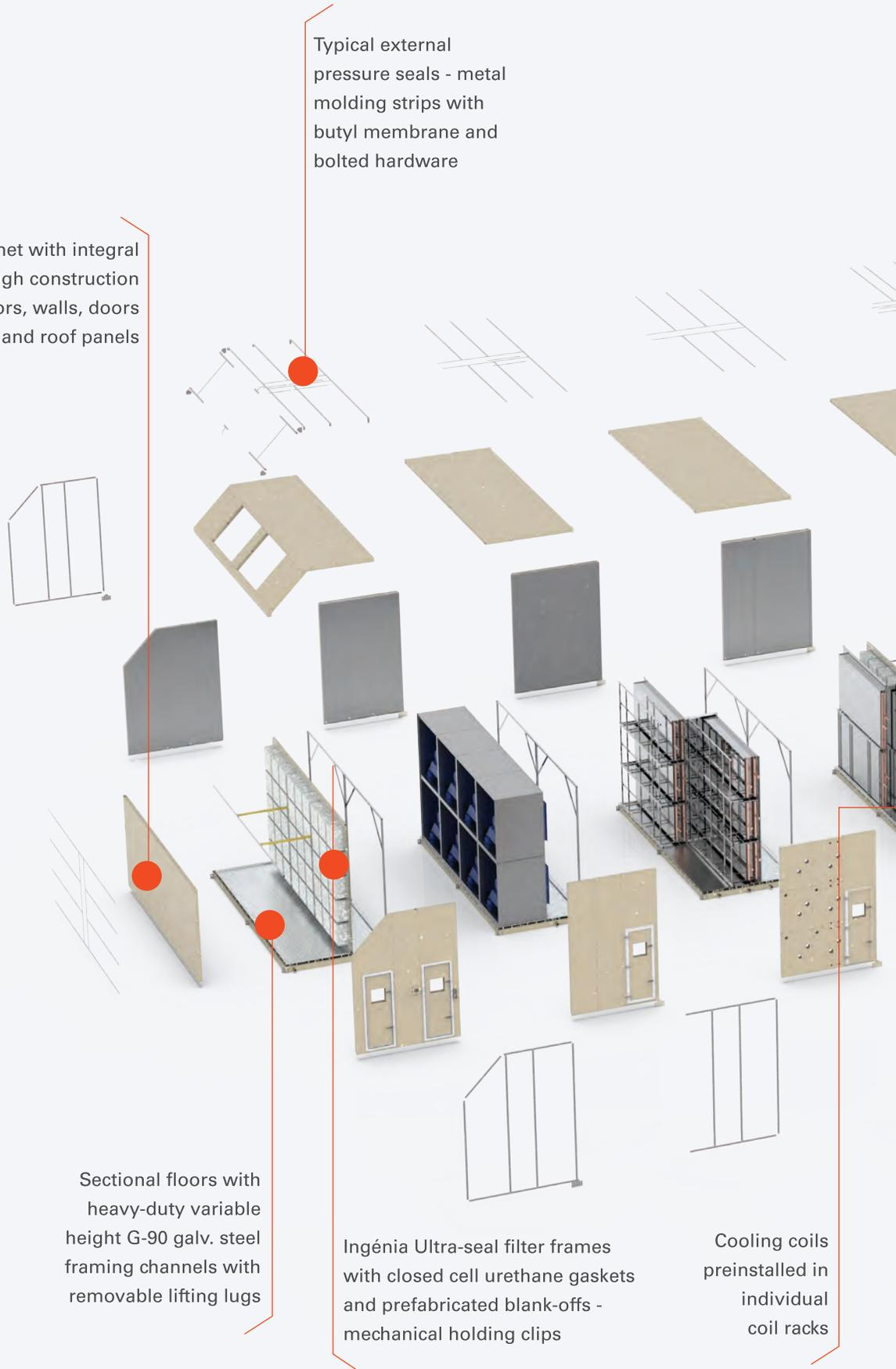
Individual fully assembled injected polyurethane foam panels with no-through metal construction
